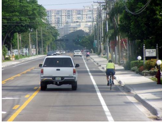
Figure 33 A converted four-lane roadway to three-lane roadway (44)
